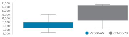
The first chart compares actual first run cyclic interval data for V2500-A5 and CFM56-7B engines.
