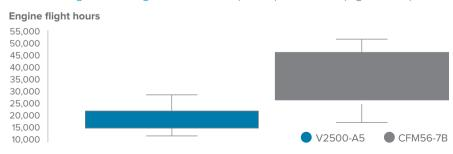
The flight hour depiction reveals much the same. On the CFM56-7B, a further revelation is perhaps the longevity of the engine when operating at larger flight hour to flight cycle ratios compared with OEM indications and V2500-A5 engines (note that in many of these instances with long on-wing time, first run engine shop visits included an LPT workscope). As with the cycle view, we again see that the V2500-A5 is more consolidated and managed around LLP replacements at the second shop visit.
