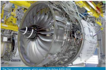
The Trent XWB=97 engine, which powers the Airbus A350-1000
